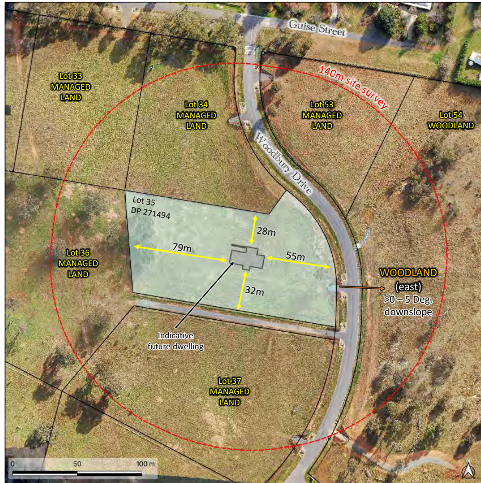
Figure 7 – RPAS aerial image captured 13.6.24, showing Woodland hazard to the east. (Dau, 2024, modified TANX Environmental, 2024)
