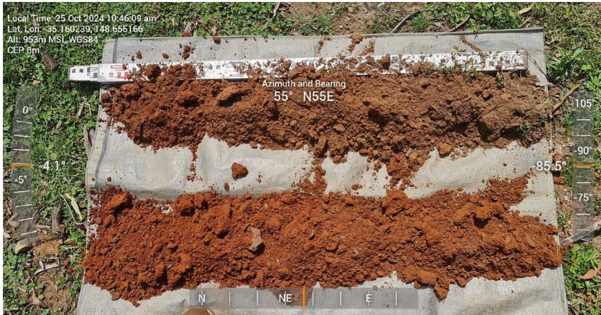
Figure 27: Soil profile 1 Building Envelope Lot 1
