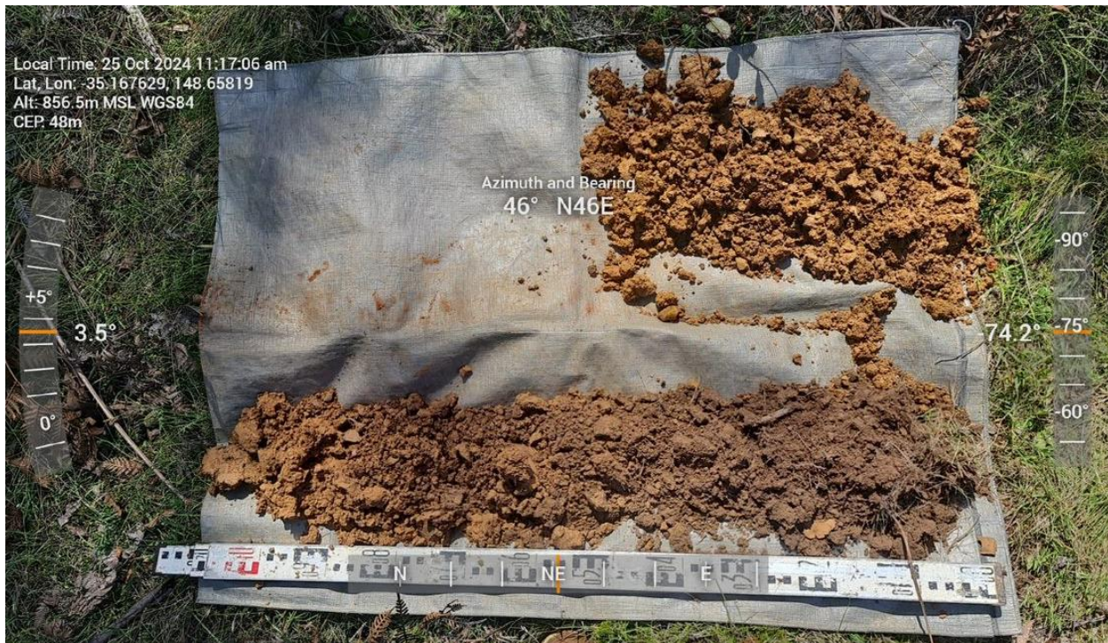
Figure 28: Soil profile 2 - Building Envelope Lot 2
