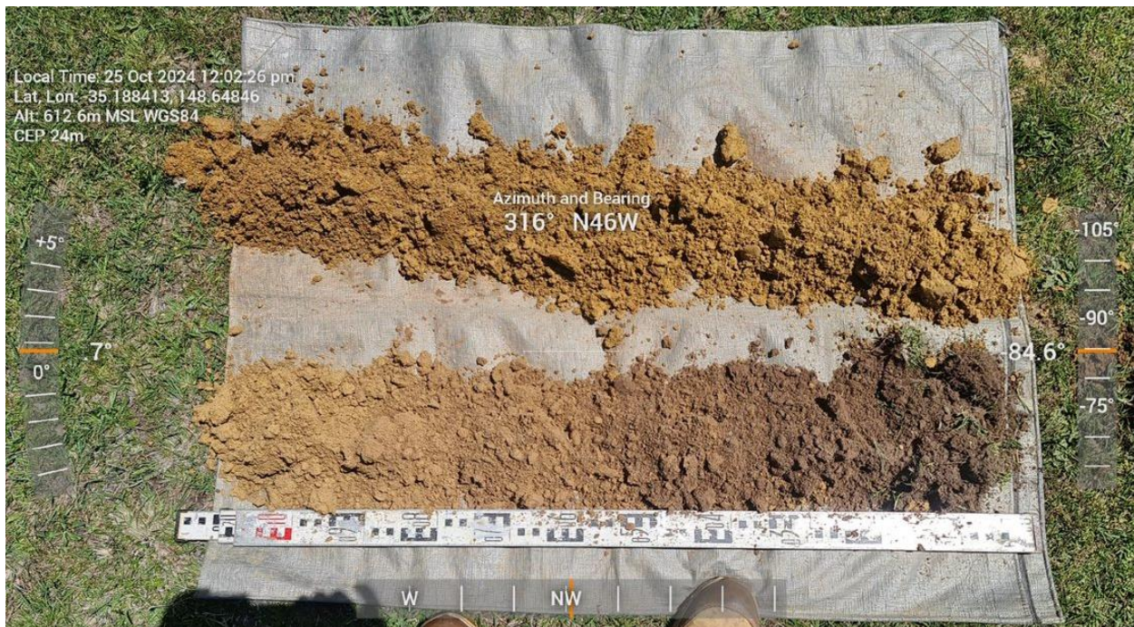
Figure 30: Soil profile 4 - Building Envelope Lot 4
