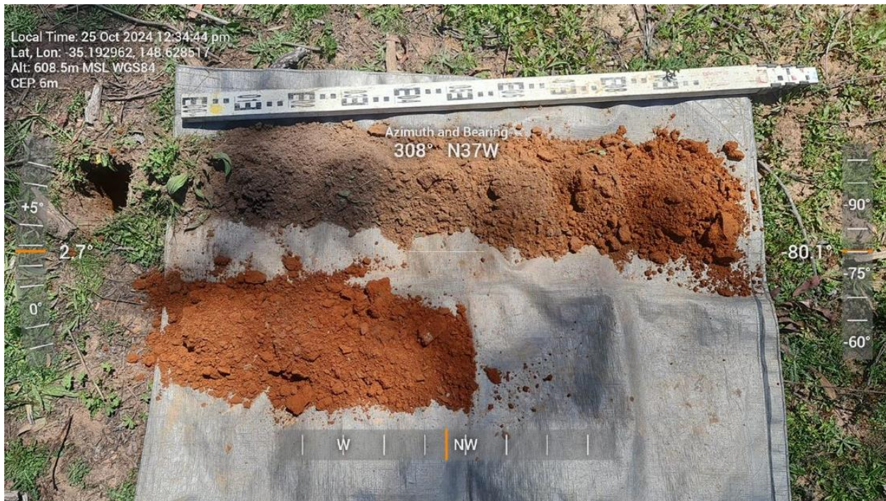
Figure 29: Soil profile 3 - Building Envelope Lot 3
