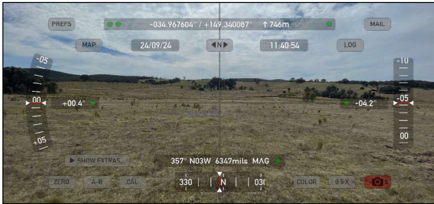
Figure 19 – Photo showing 0.5° downslope to the north (McGregor,2024)
