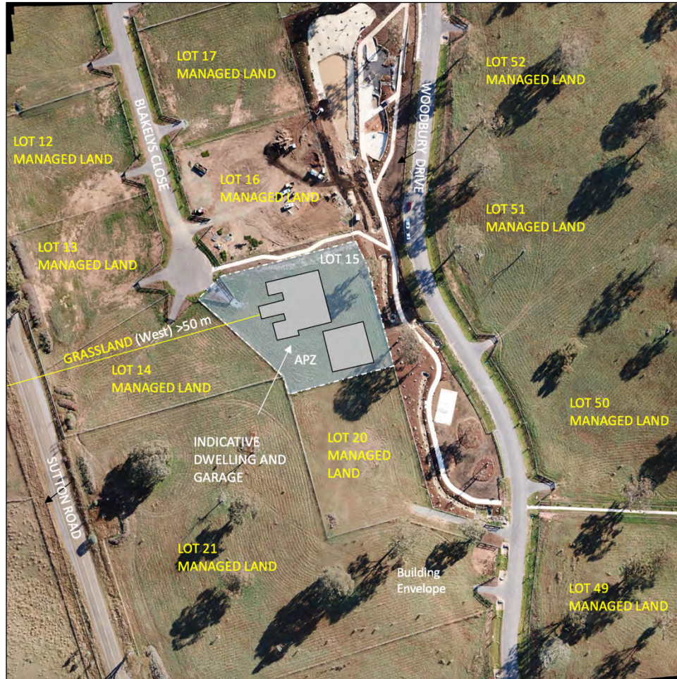
Figure 7 – RPAS aerial image captured 14.5.24 showing closest hazard (grassland) greater than 50 m from the Subject Lot resulting in BAL-LOW outcome. (Dau, 2024)
