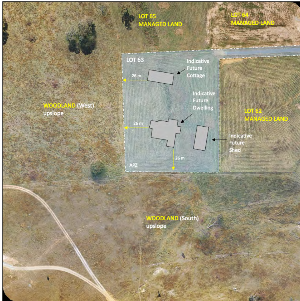
Figure 7 – RPAS aerial image captured 30.4.24 Showing vegetation formations, slope, and indicative APZ setback distances. Not to scale. (Dau, 2024)
